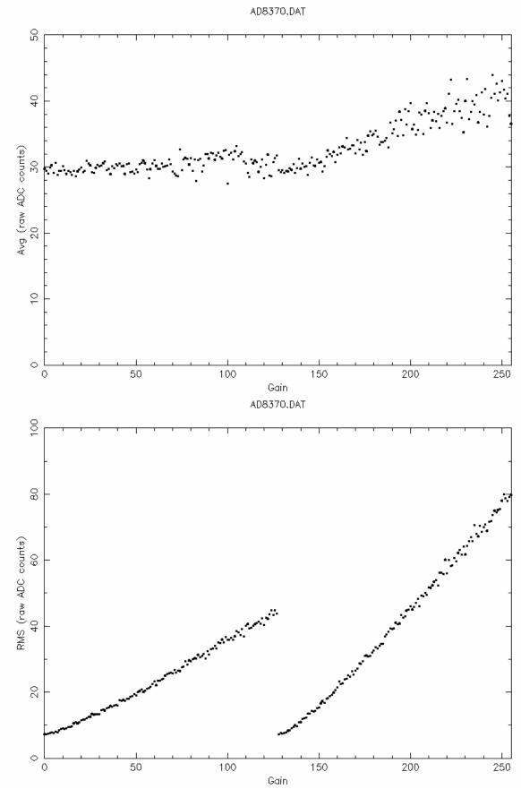
Note: Each measurement point corresponds to data taken over 1024 turns for 1 bunch on channel 0; channel 0 terminated with a 50 Ohm resistor
