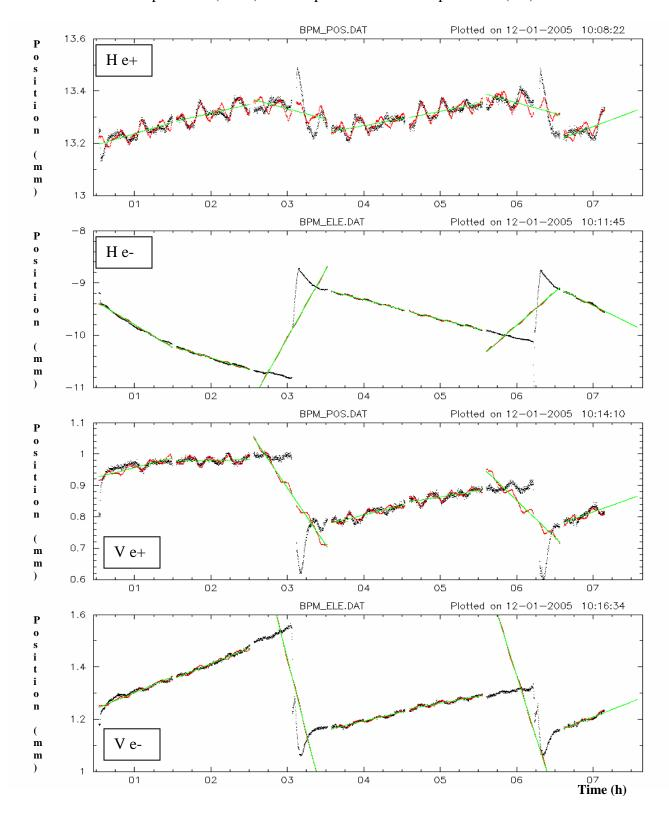
"Raw" positions (black) and temperature based compensation (red) over  $\sim 1$  hour
