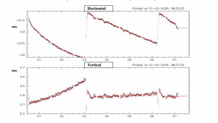
Position differences (electron - positron): "raw" (black) and temperature compensated (red) over ~ 1 hour
