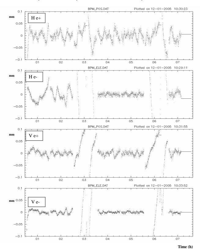
Temperature based compensation subtracted from "raw" positions over ~ 1 hour
