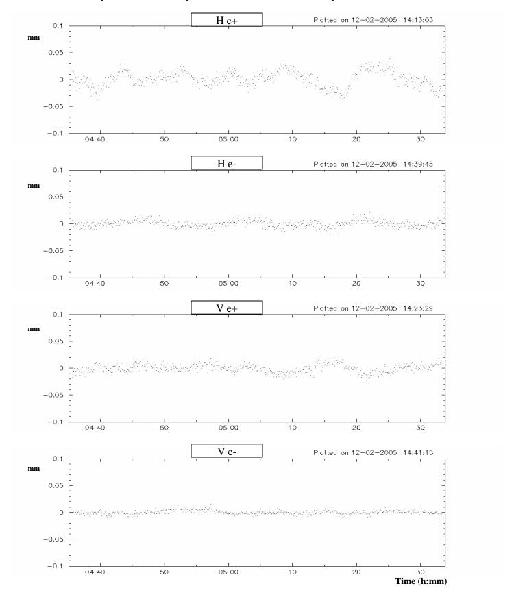
Position differences (electron - positron): "raw" (black) and temperature compensated (red) over ~ 7 hours
