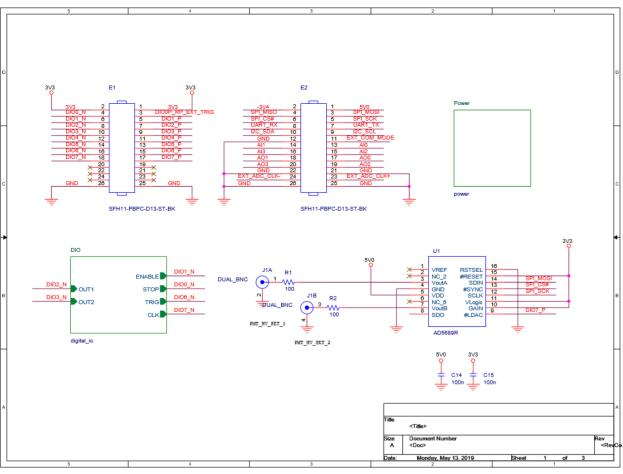
SCHEMATIC 1 - DAC & Expansion Slot Schematic
