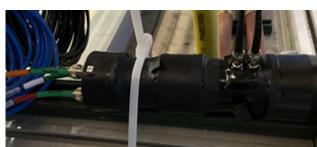
Figure 4 - PMT tie-wrapped to Girder
