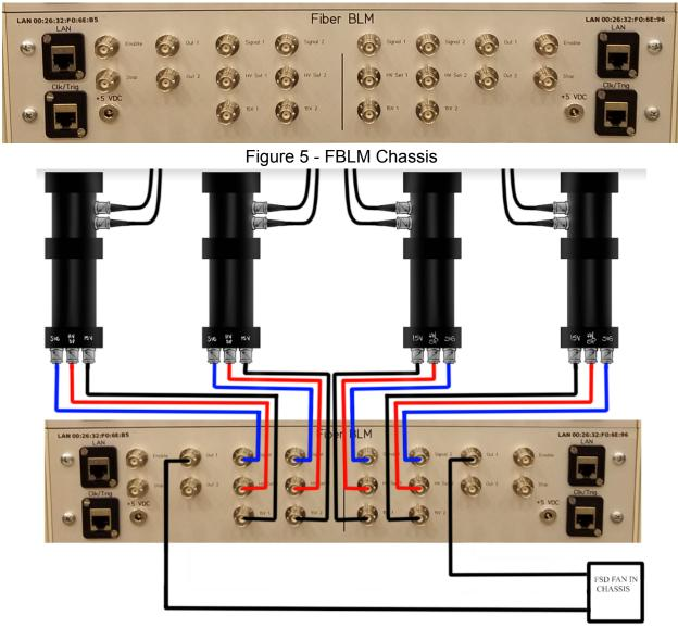
Figure 6 - FBLM Chassis wired to four PMTs and Fast Shut-Down(FSD) FAN IN Chassis
