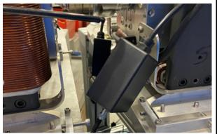
Figure 3 - PMT Fiber Interconnect Box
