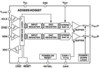
Figure 11 - AD5689 Functional Block Diagram
