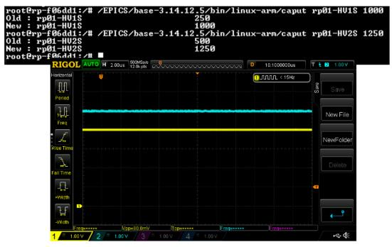
Illustration 2 – DAC 1 set to 1000 / DAC 2 set to 1250 (Scope Setting: 1V/DIV; DAC 1 = 4V, DAC 2 = 5V)
