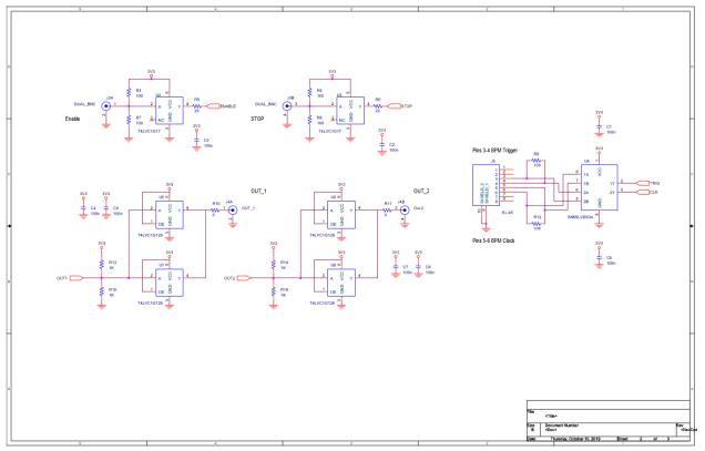
SCHEMATIC 2 - Trigger/Clock/Buffer, Expansion Board
