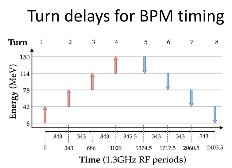
Number of RF periods between turns for a single bunch making 8 passes through the MLC, traversing through all of the acceleration and deceleration energies. Note that the number of periods between turns 4 and 5 is 2.5 more than the others. This is where the beam passes through splitter 4, which has a longer path length.
