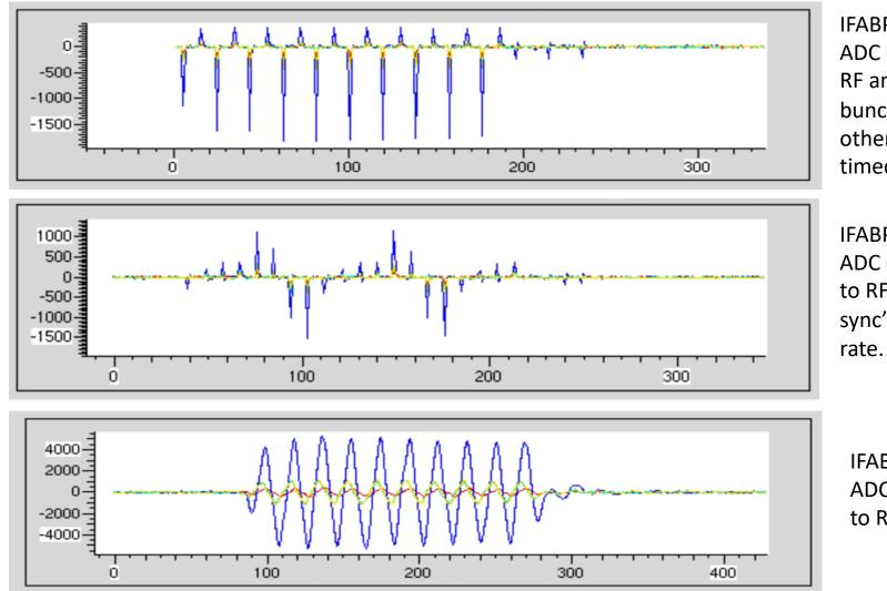
IFABPM02 ADC clock locked to RF and sync'd to bunch rate. Every other bunch is timed to peak.
