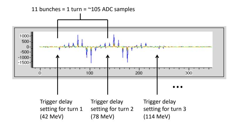
Trigger delay timing will be changed to set the start ADC sample for the selected energy, and the number of ADC samples used for each energy is ~100 or one full turn.
