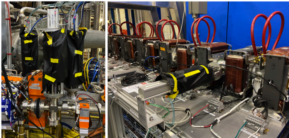
Figure 2.8-20: Three view screens at end of R1, R2, and R3 lines (left) and view screen installed in FFA loop (right).
