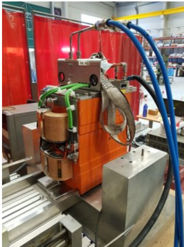
Figure 2.3-3: Splitter dipole magnet on the measurement system at Elytt Energy. The narrowed “waist” and the shaped chamfer on the end of the bottom pole face are in evidence.
