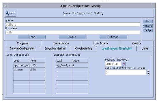
FIGURE 7-4 Queue Configuration—Load Thresholds
