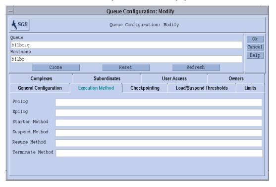
FIGURE 7-2 Queue Configuration—Execution Method parameters
