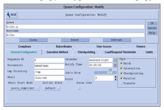
FIGURE 7-14 Calendar Configuration in General Parameters Queue Configuration Menu
