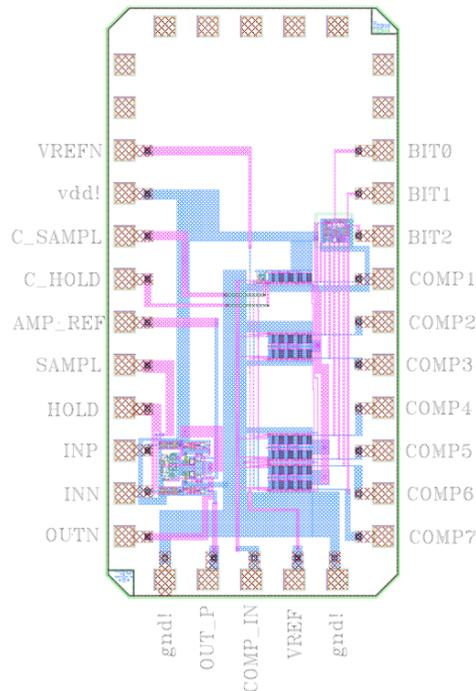
Figure 3. Picture of a 3-bit cell.
