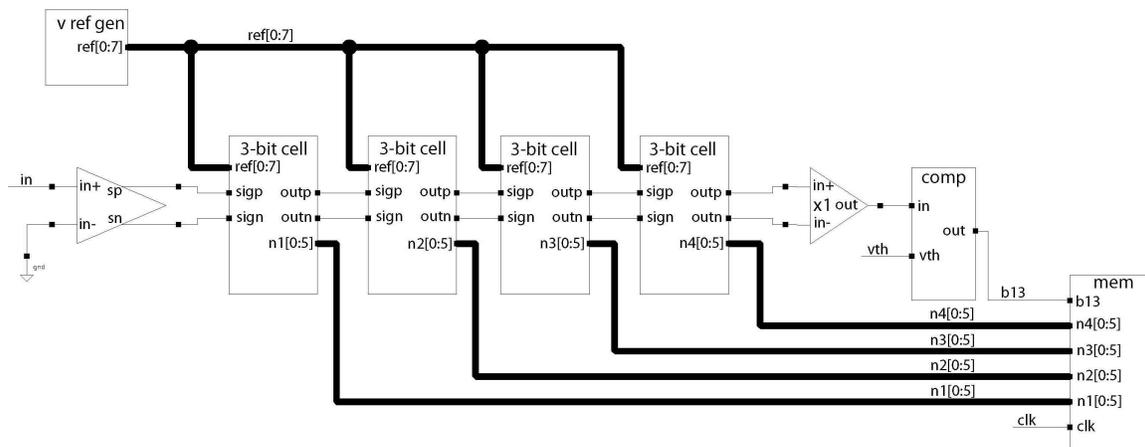
Figure 1. Schematic of a 12-bit pipelined digitizer.
