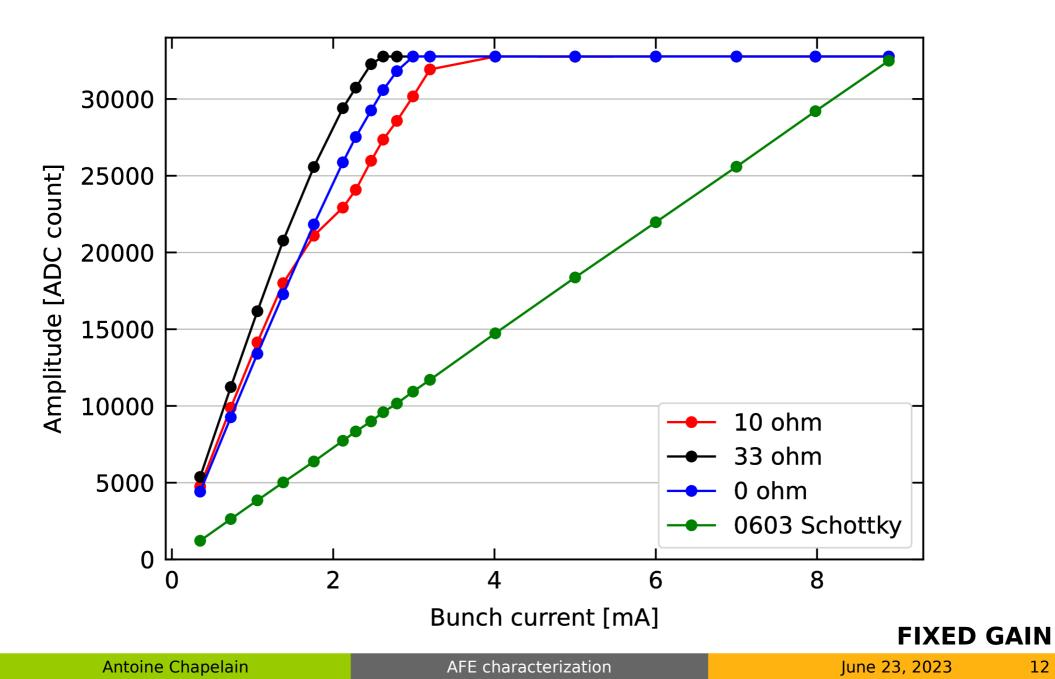
0 ohm and Schottky gains scaled to match 33 ohm at low current
