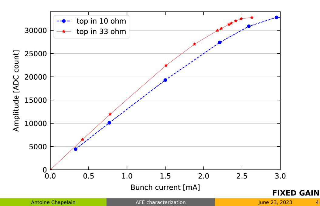
10 ohm gain scaled to match 33 ohm at low current
