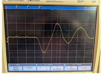
400 milli-volts pk-pk into 50 ohm load after 1:6 splitter, 2960 ps positive peak to negative peak
