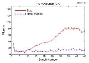
Figure 3. Bunch by bunch beam size and rms motion at 14ns spacing, 1mA/bunch, 45 bunches. The beam profile is measured with the xray beam size monitor. Blowup first appears in bunch 10. Blowup of the first bunch is not well understood.
