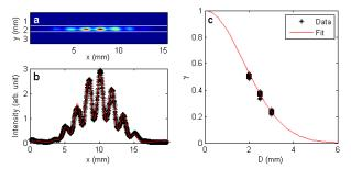
Figure 5. (a) A typical interference pattern of SR using a D=2.0 mm double slits. (b) The horizontal intensity profile integrated between two white lines in (a) and the best fit. (c) The visibility measured using three different sets of double slits (D = 2.0, 2.5, and 3.0 mm). The red line is the best fit.
