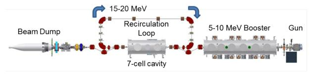
Figure 9. The compact energy recovery recirculation loop concept. The existing photoinjector, a cryomodule containing one 7-cell SRF cavity, and high power beam stop will be used to recirculate up to 100 mA beam current at 15-20 MeV beam energy.
