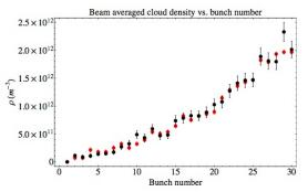
Figure 2. Average initial (before the "pinch") electron cloud density vs. bunch number, comparison between estimate from measured tune shifts (red) and, simulation (black) from POSINST.
