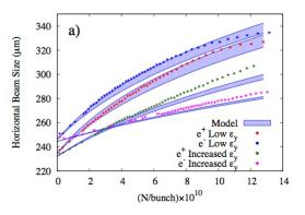
Figure 4. Horizontal beam size vs particles/bunch. Points are data. Band is the theory. The width of the band corresponds to the uncertainty in measurement of the "zero" current vertical beam size.
