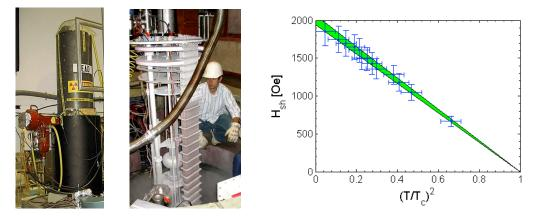
Figure 8. Left: 1.5 MW pulsed klystron. Middle: Graduate student Nick Valles with his waveguide insert for pulsed operation of single-cell SRF cavities at high power. Right: Measured temperature dependence of the superheating critical field of niobium.
