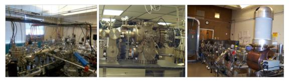
Figure 7: Cornell photocathode research facilities. Multipurpose cathode chamber (left), dedicated MBE growth reactor (center), photoemission gun with diagnostics (right). Photocathodes under UHV can be moved between these chambers.
