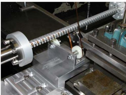
Figure 4: Undulator winding on a lathe.
