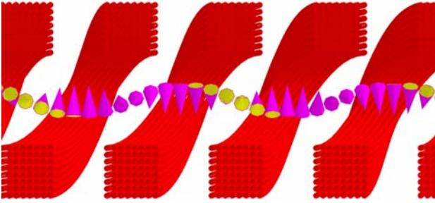
Figure 1: 3d OPERA multiwire model of the undulator. Cones represent the magnetic field vector.
