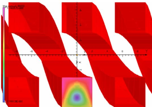
Figure 2: Region with highest peak field (pink coloured) in the undulator winding.
