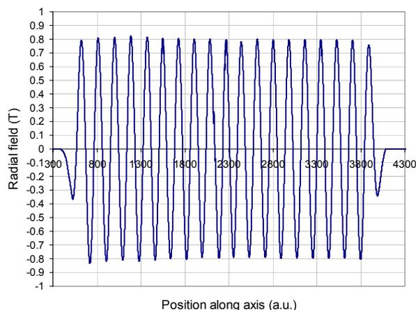
Figure 6: Profile of the axial component of the magnetic field on the undulator axis.
