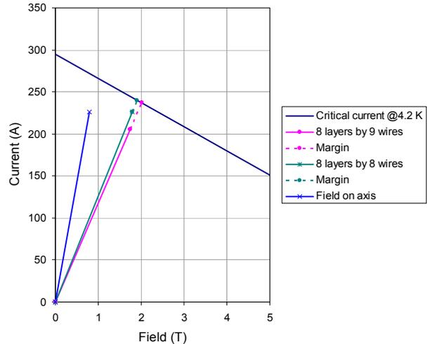
Figure 3: Undulator conductor load lines.
