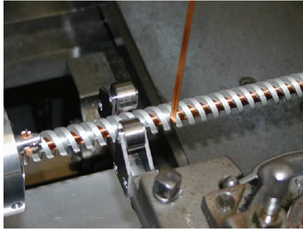
Figure 5.5: Undulator prototype with super-conducting (SC) wires being wound [193].
