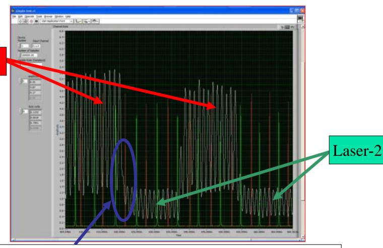
Chopper edge effects and low photodiode duty cycle per laser complicate measurement – requires study
