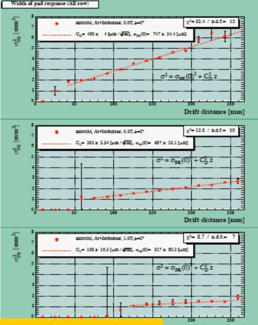
Measured C<sub>D</sub> in good agreement with Magboltz Simulation Prift distance [mm]
