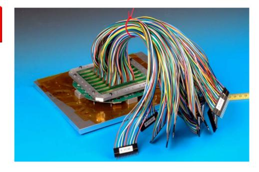
June 6th: Re-assemble, test with <sup>55</sup>Fe in Ar+5%isobutane, OK, connect pad electronics. **See tracks!** Take data overnight
