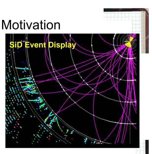
But we do have a finely segmented EM calorimeter – can start from there, using MIP stubs as seeds.
