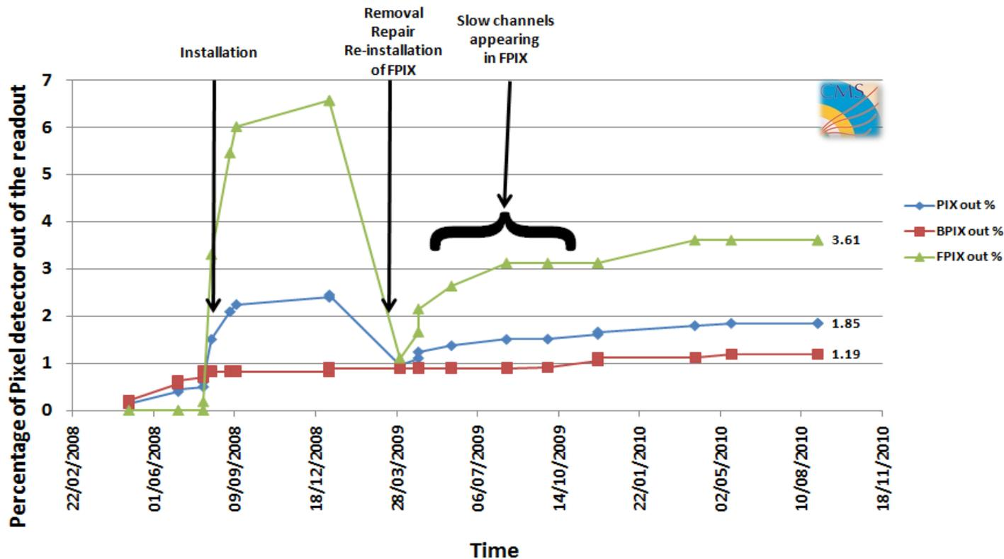
CMS demonstrated that the pixel detector could be removed, repaired, and reinserted in a period of 3 months.
